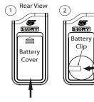
1. Slide the battery cover up by applying equal pressure at its top and bottom (the arrow on the cover indicates the direction), remove the cover from the remote control housing.
